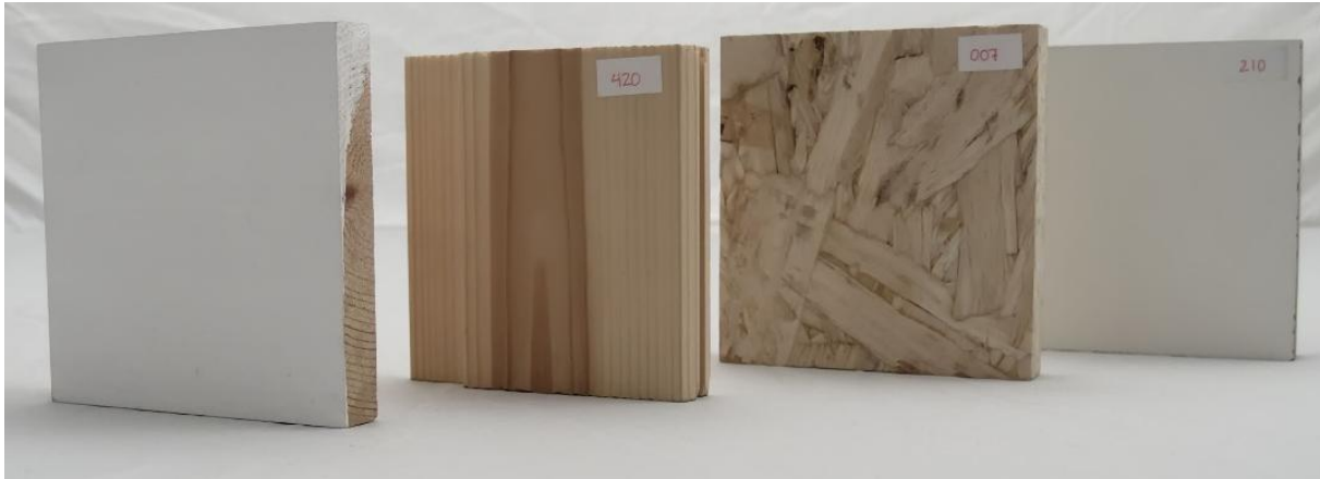
Figure 1. Material samples used in focus groups. From left to right: painted pine, knot-free pine tongue and groove decking, oriented strand board (OSB), and medium density fibreboard (MDF)
