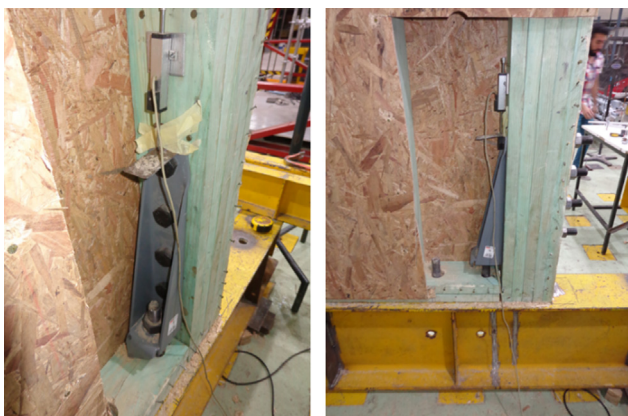
Fig. 3. Sturdy end studs hold-down anchorage.
