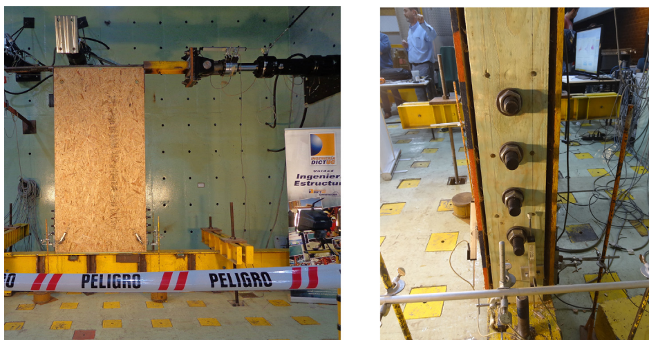
Fig. 3. Test setup (front and right view) for a 1200 mm long strong wall, labelled as C120-10-01 by Guíñez et al. [6].
