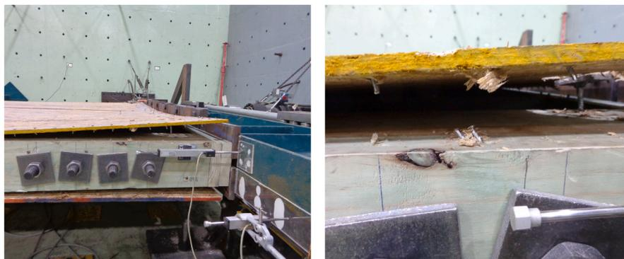
(a) Shear- and bending-failure of the nails in panel (b) Panel crushing due to the progressive damage of edges.
