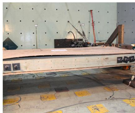
(c) Panel buckling due to the contact between the panels and the steel beams at large displacements.
