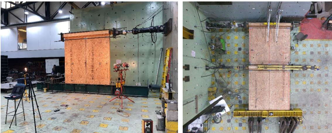
Figure 3. Shear walls tests specimens with A.T.S., one story test (Left), two stories test (Right).
